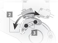
Tighten screws to lock plate in position.
