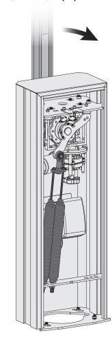
· Springs installed on the left side
