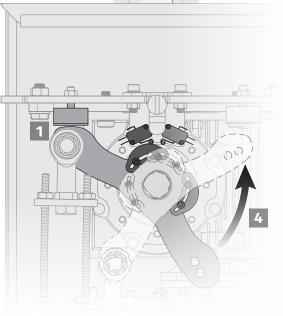
When the opening or closing micro switch is activated, check if the respective LED on the control board turns off.
