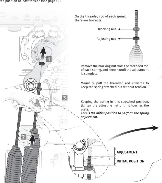
Hold the threaded rod with a pliers so that it does not rotate, and keep tightening the adjusting nut until each spring is stretched the distance mentioned in the table on page 15.
